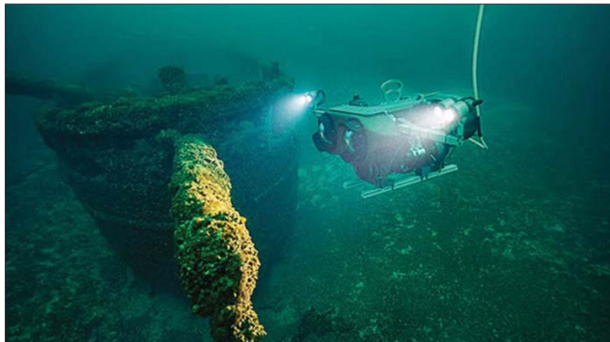
An ROV – Remote Operated Vehicle – exploring and documenting the remains of a sunken wooden schooner. Courtesy N.O.A.H.
